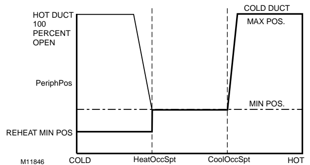
Fig. 36. Heat/Cool Modes for Dual Duct, Pressure Dependent cooling and heating, with Flow mixing and no flow pickups.
